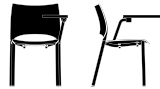
1716 Armless chair, molded nylon seat and back, Tablet Left Sitting W 24.75" D 22.5" H 32.75" SH 17.5" TH 28.5"
